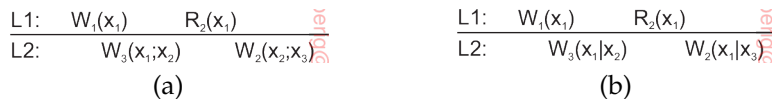
Figure 7.19: (a) A writes-follow-reads consistent data store. (b) A data store that does not provide writes-follow-reads consistency.
