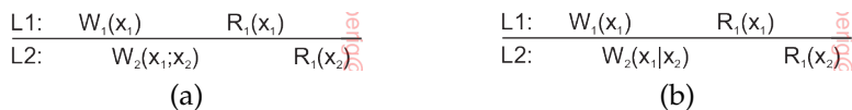
Figure 7.16: The read operations performed by a single process P at two different local copies of the same data store. (a) A monotonic-read consistent data store. (b) A data store that does not provide monotonic reads.
