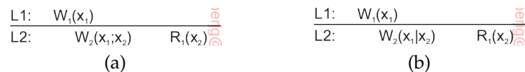
Figure 7.18: (a) A data store that provides read-your-writes consistency. (b) A data store that does not.
